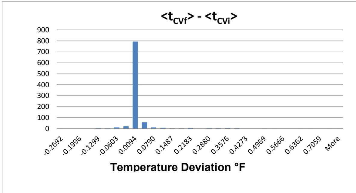
Graph 2. Distribution of temperature deviations at the start of a flow measurement and at the end of the flow measurement on the 50 gpm piston prover
