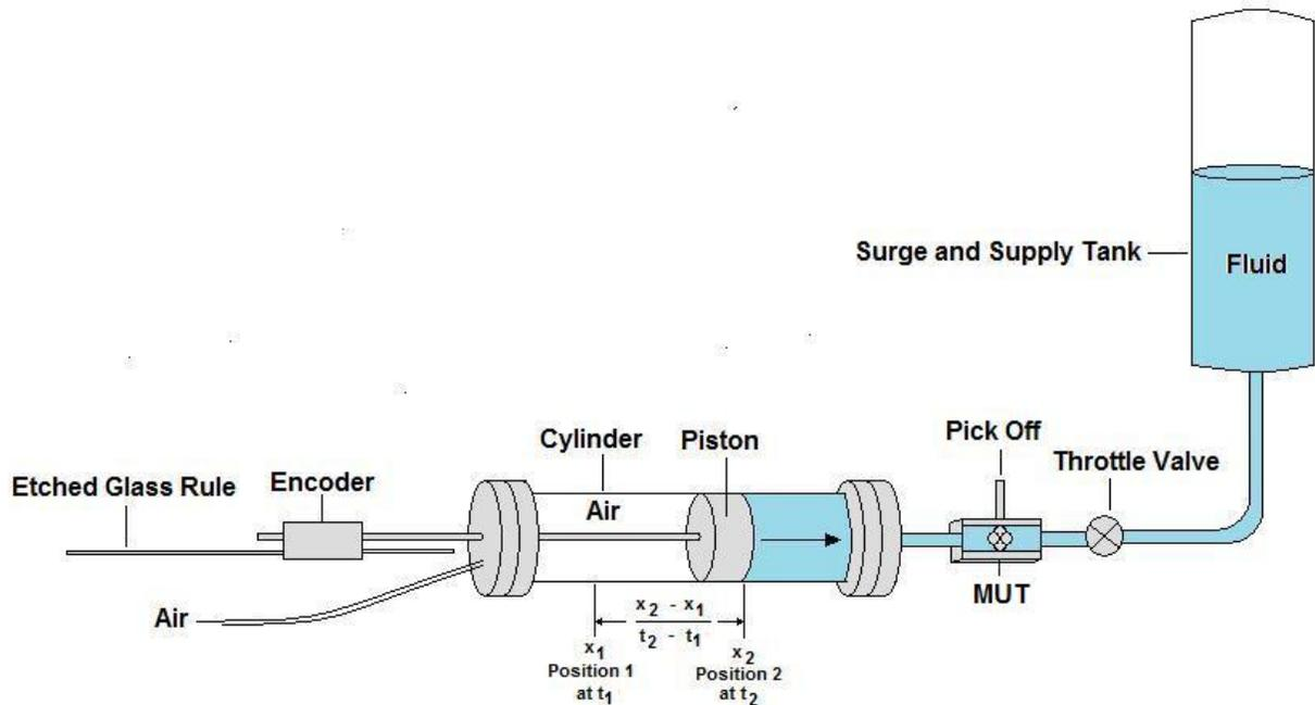
Figure 1. Simple Schematic of a Positive Displacement Piston Prover
