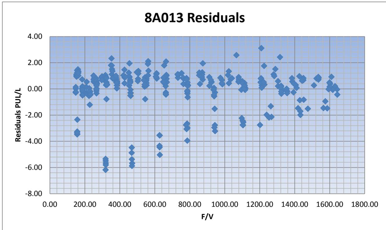
Graph 5. Scatter Plot of Turbine Flow Meter SN: 8A013 Residuals of 5 calibrations performed over 5 years
