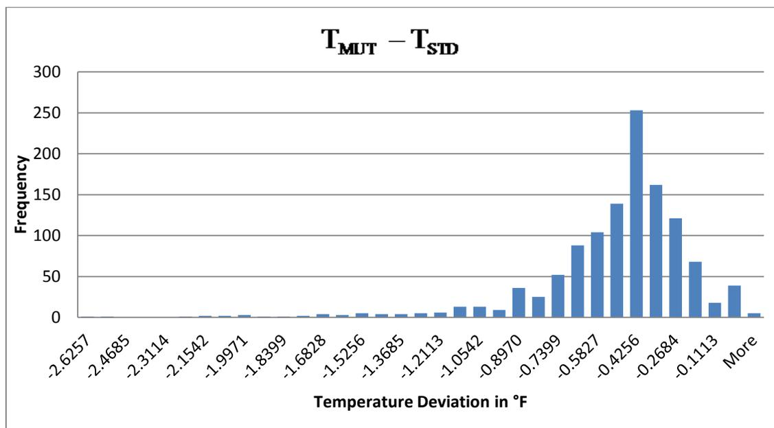
Graph 1. Distribution of Temperature Deviations between  $\bar{T}_{MUT}$  and  $\bar{T}_{STD}$  on a 10 gpm piston prover.
