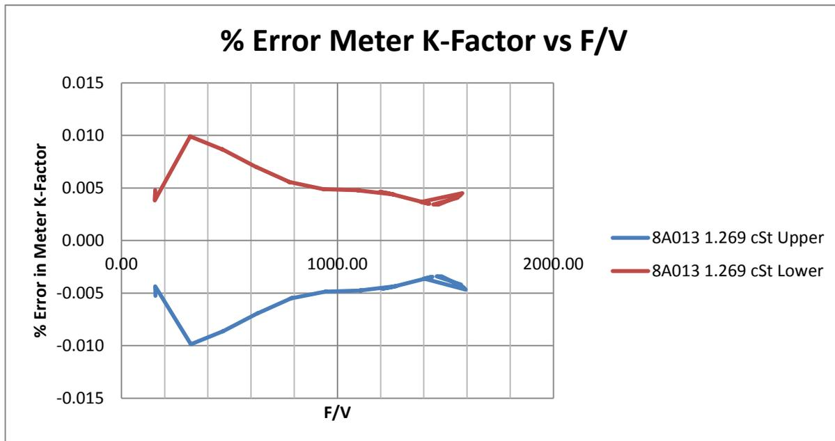
Graph 9. Plot of % Meter K-Factory vs F/V for Meter SN: 8A0131 at 1.269 cSt.
