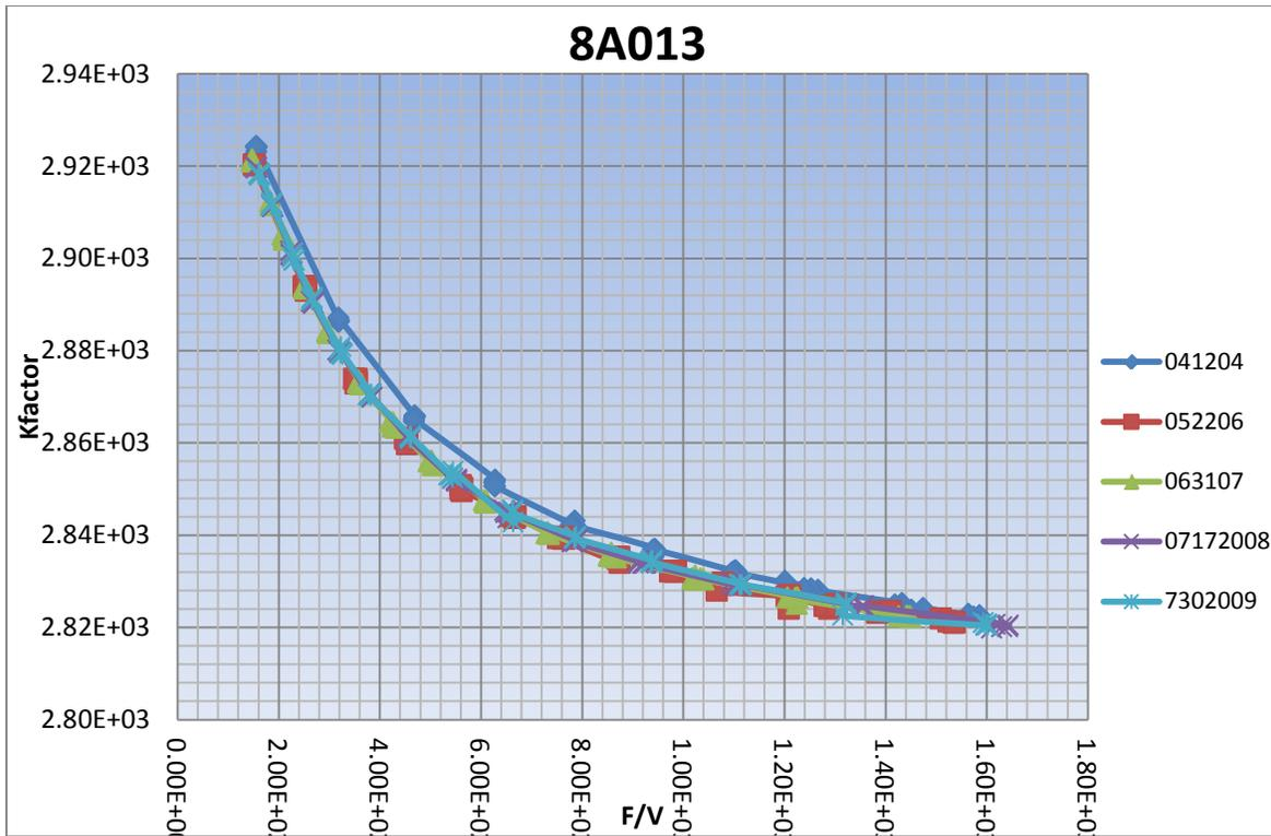
Graph 3. Calibrations of Turbine Flow Meter 8A013 over 5 years
