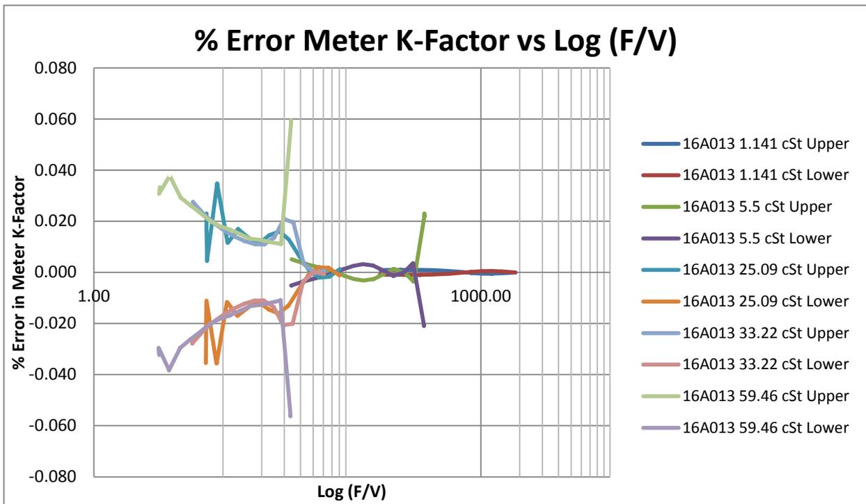
Graph 8. %Error in Meter K-Factor vs Log(F/V) for Meter SN: 16A013 at 1.14 cSt, 5.5 cSt, 25.09 cSt, 33.22 cSt, and 59.46 cSt.
