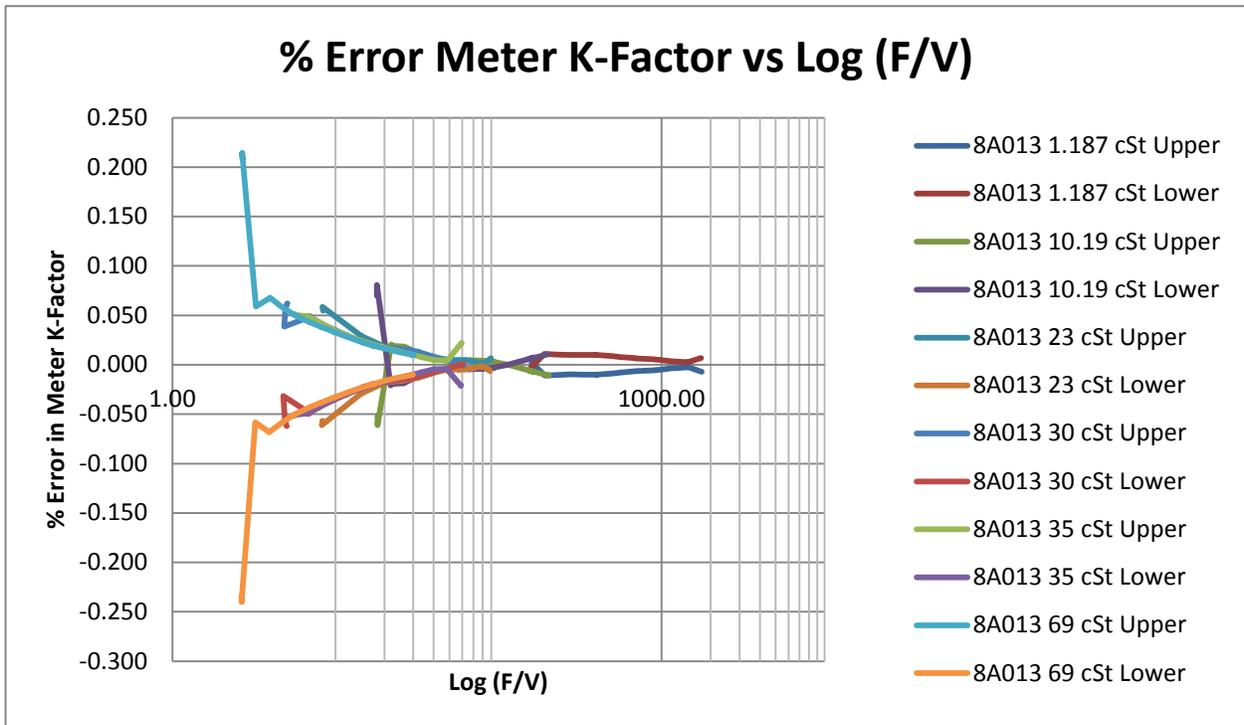
Graph 7. %Error in Meter K-Factor vs Log(F/V) for Meter SN: 8A013 at 1.187 cSt, 10.19 cSt, 23 cSt, 30 cSt, 35 cSt, and 69 cSt.
